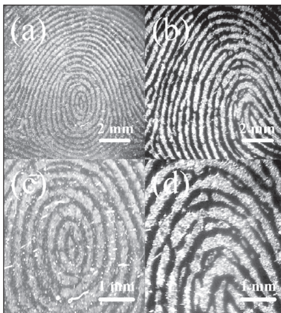
Fig.1 Representative sputter coated latent prints on a glass surface a) and b): Latent prints showing 1 st and 2 nd level detail. c) and d): close up views of developed latent prints showing 2 nd and 3 rd level detail.
