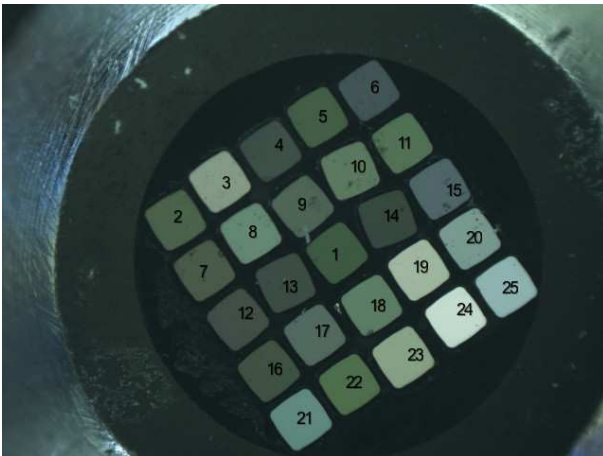
Figure 2. Left: The square-core bundle tested in this paper. Each of the 25 fibres have 195 \times 195 \mu\text{m} cores. The fibres are separate on output and only bundled for the first few centimetres. Right: One of the 61-core fused hexabundles used in the SAMI instrument. The cores are 105 \mu\text{m} in diameter.
