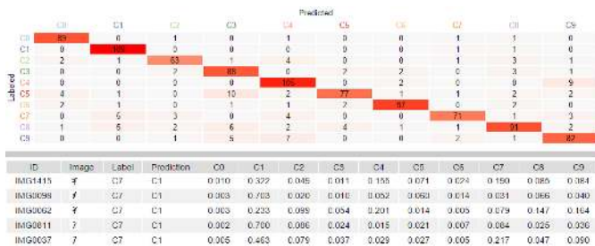
Fig. 7. The interactive confusion matrix used in our controlled study. Each cell shows instance counts and is color-coded by the number. Selecting cells, columns or rows reveals selected instances in the adjacent sortable table (below the matrix).
