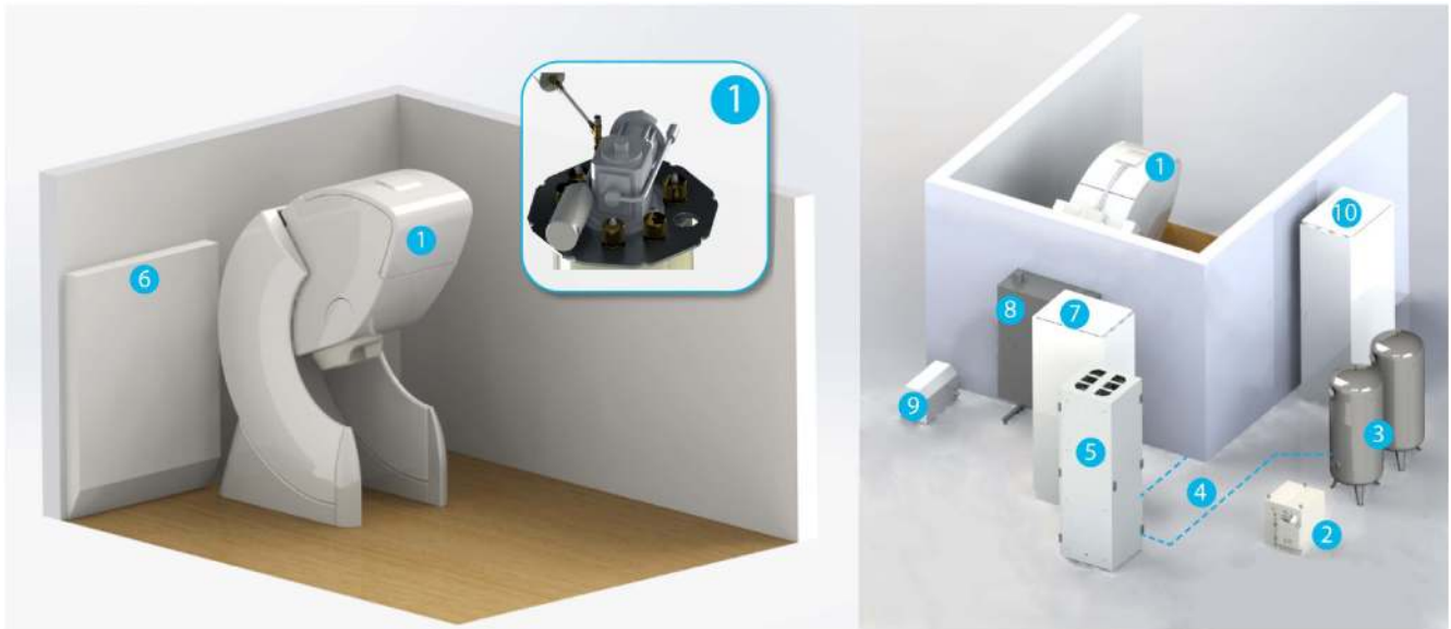
Figure 17. Internal helium recycling system (Elekta Oy). (1). Cryocooler cold head is inserted in the top part of the dewar in the MEG probe unit inside the magnetically shielded room. (2). Cryocooler compressor. (3). Storage tanks. (4). Helium gas lines. (5). Helium recycler cabinet. (6). Reel for cryocooler hoses. (7). MEG electronics cabinets. (8). MEG electronics feedthrough unit. (9). Lifting unit for MEG probe. (10). Cabinet for stimulators. Items 1–6 are parts specific to the helium recycler.
