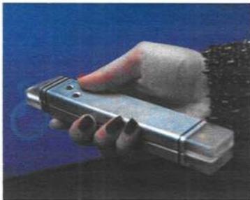
Figure 3: Well-known devices such as an omnipresent laser pointer enhanced with button module, LEDs and vibration motor provide flexible input from any distance. Users benefit from a more natural and convenient pointing experience.
