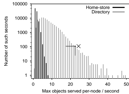
(a) Redmond: Average maximum load for a node is 1.5 objects/s and 6.6 objects/s for home-store and directory respectively.
