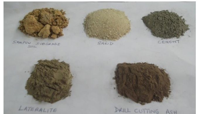
Figure 2: Soil sample, additives and binder used
