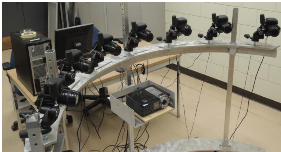
Figure 12. Multi-camera photogrammetric system consisting of seven DSLRs attached to a metal frame.
