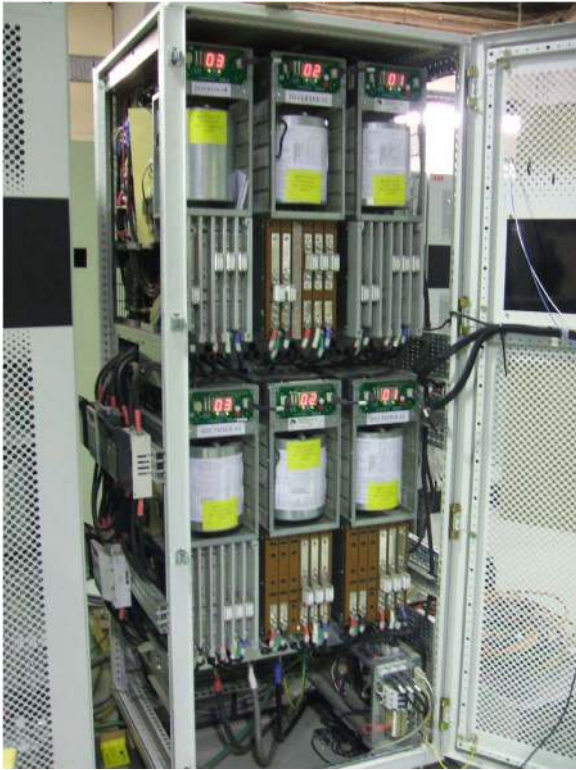
Fig. 13. Test hardware. Three pairs of reconfigurable active rectifiers and output inverters.
