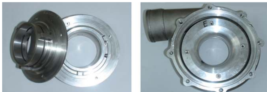
Fig. 8 Separated shroud with SRCT and volute
