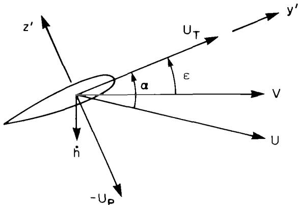
Figure 5.- Rotor blade airfoil section in general unsteady motion.
