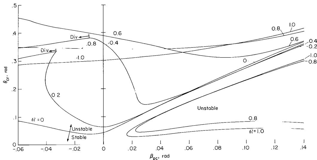
Figure 35.- The effect of  $\Omega$  on the stability boundaries,  $\theta_{cr}$  versus precone angle:  $\omega_\phi = 2.5$ ,  $\omega_v = 1.5$ .
