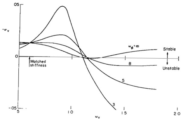
Figure 42.- The effect of torsion frequency on lead-lag modal damping versus lead-lag frequency:  $\beta_{pc} = 0.0$  rad,  $\theta = 0.3$  rad,  $R = 0.0$ .
