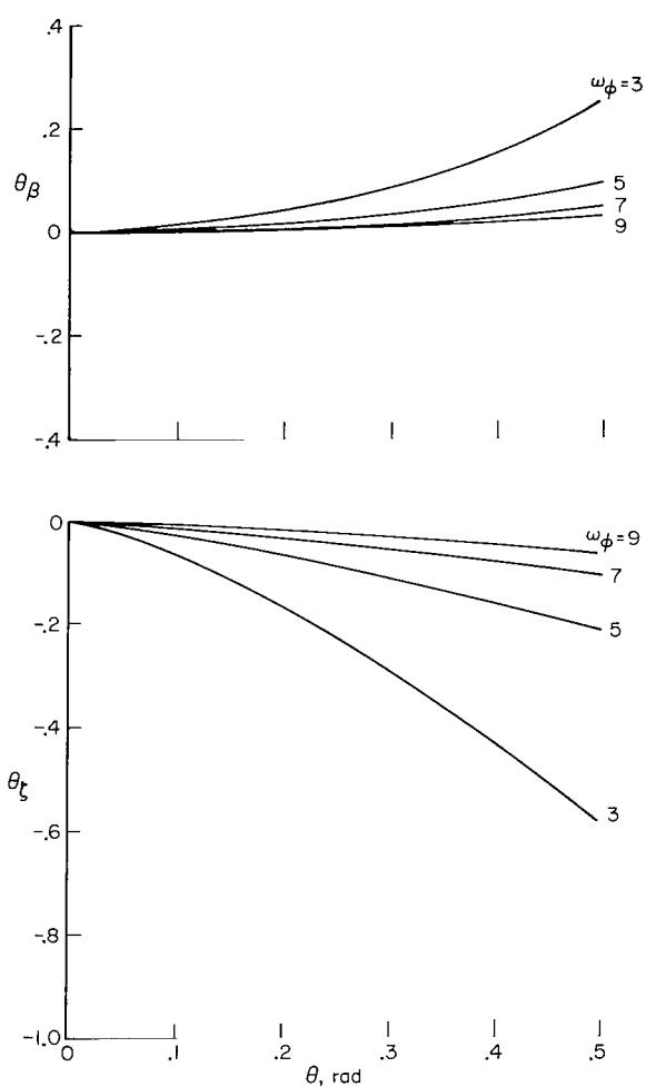
Figure 15.- Equivalent pitch-flap and pitch-lag coupling for a soft inplane rotor blade:  $\omega_v = 0.7$ ,  $\mathcal{R} = 0.0$ ,  $\beta_{pc} = 0.0$  rad.
