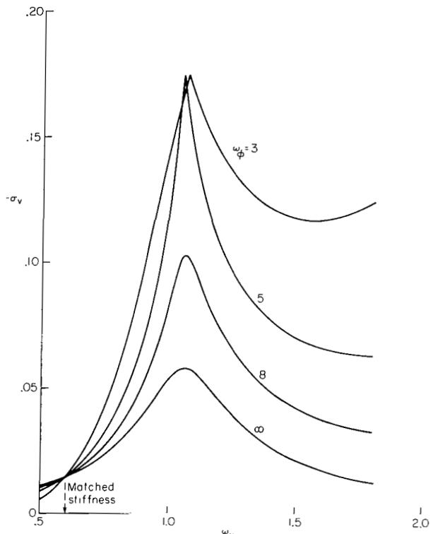
Figure 44.- The effect of torsion frequency on lead-lag modal damping versus lead-lag frequency:
