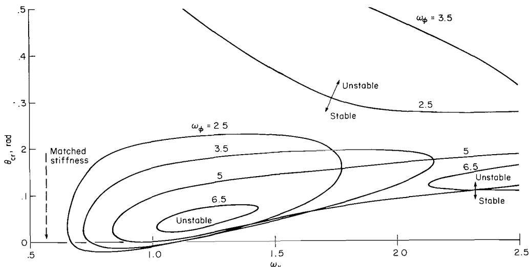
Figure 33.- The effect of precone and torsion frequency on the stability boundaries,  $\theta_{cr}$  versus lead-lag frequency:  $\beta_{pc} = 0.1$  rad,  $R = 1.0$ .
