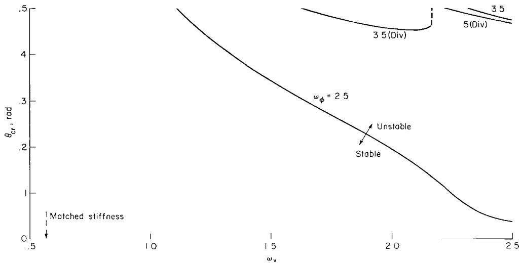
Figure 27.- The effect of torsion frequency on the stability boundaries,  $\theta_{cr}$  versus lead-lag frequency:  $\beta_{pc} = 0.0$  rad,  $\mathfrak{R} = 0.8$ .
