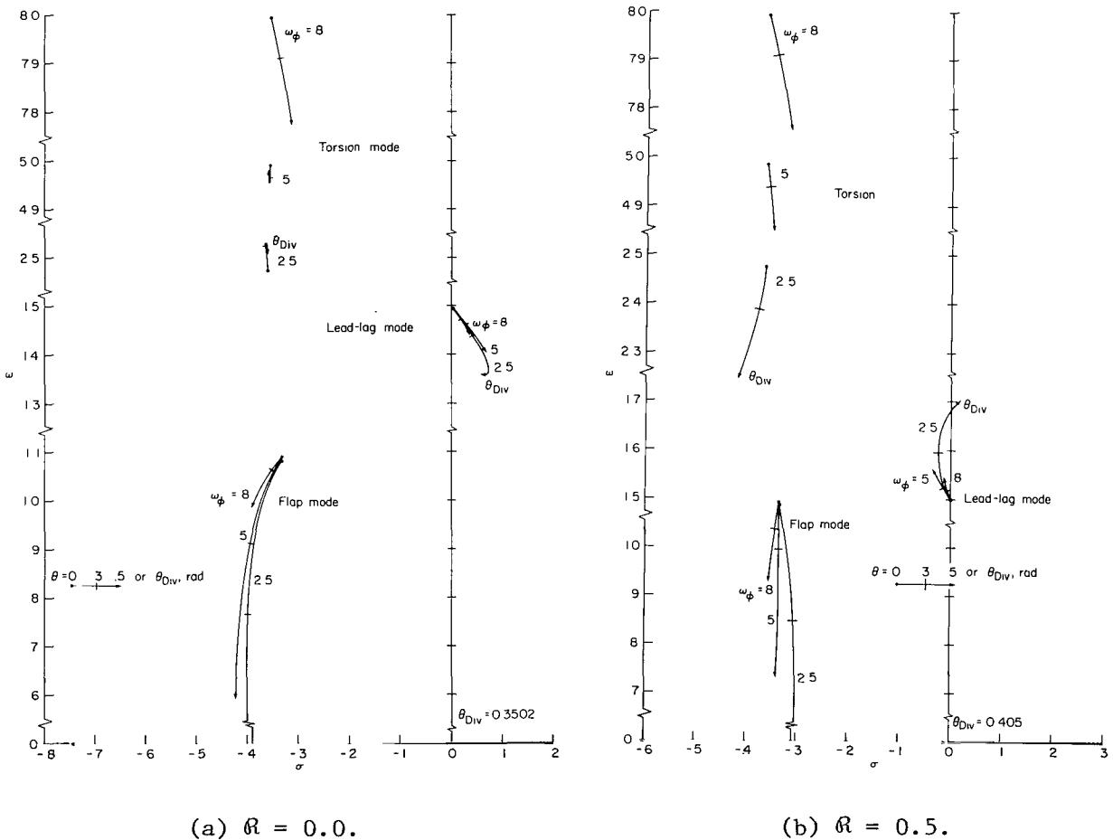
Figure 21.- Locus of roots for stiff inplane rotor blade:  $\omega_v = 1.5$ ,  $\beta_{pc} = 0.0$  rad.
