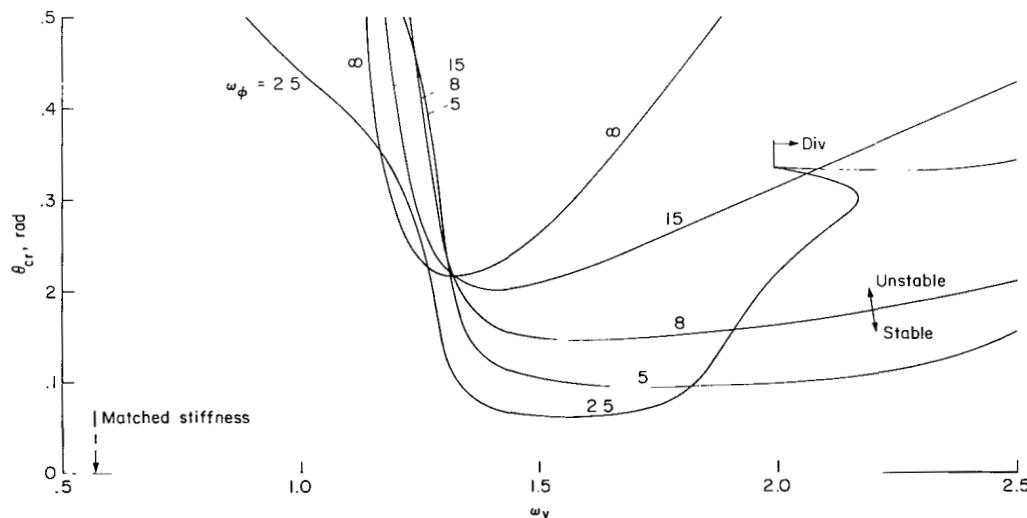
Figure 24.- The effect of torsion frequency on stability boundaries,  $\theta_{cr}$  versus lead-lag frequency:  $\beta_{pc} = 0.0$  rad,  $\Re = 0.2$ .
