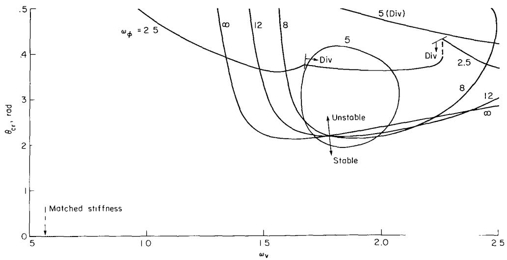
Figure 25.- The effect of torsion frequency on the stability boundaries,  $\theta_{cr}$  versus lead-lag frequency:  $\beta_{pc} = 0.0$  rad,  $R = 0.4$ .
