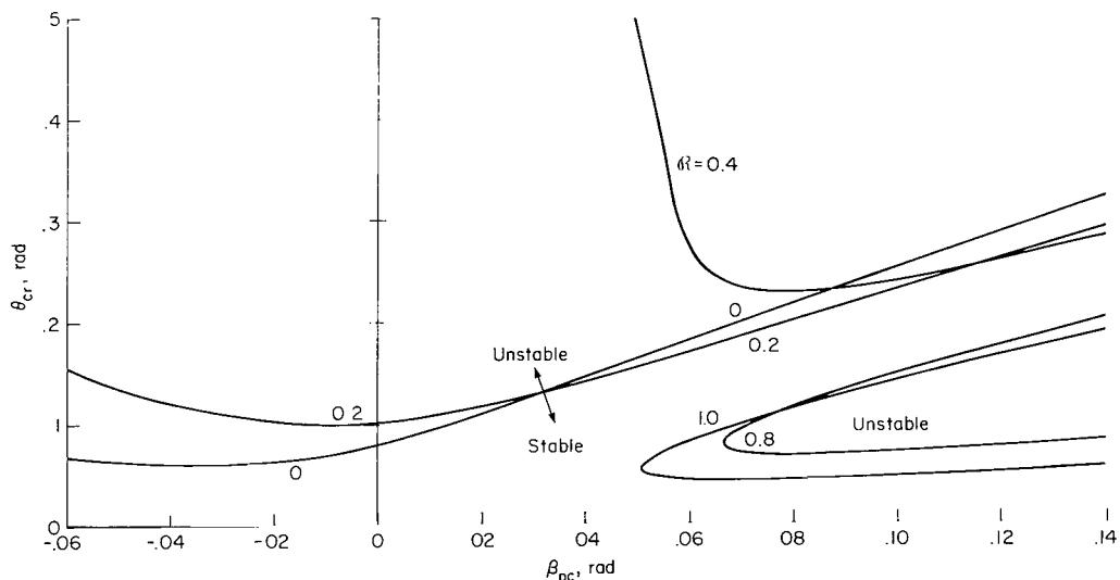
Figure 36.- The effect of  $\Omega$  on the stability boundaries,  $\theta_{cr}$  versus precone angle:  $\omega_\phi = 5.0$ ,  $\omega_v = 1.5$ .
