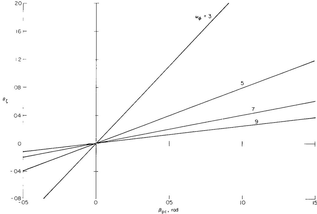
Figure 14.- The effect of torsion frequency and precone on the equivalent pitch-lag coupling for zero pitch angle:  $\omega_v = 0.7$ ,  $\mathcal{R} = 0.0$ ,  $\theta = 0.0$  rad.
