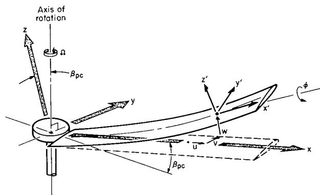
Figure 3.- Rotor blade coordinate systems and deflections.
