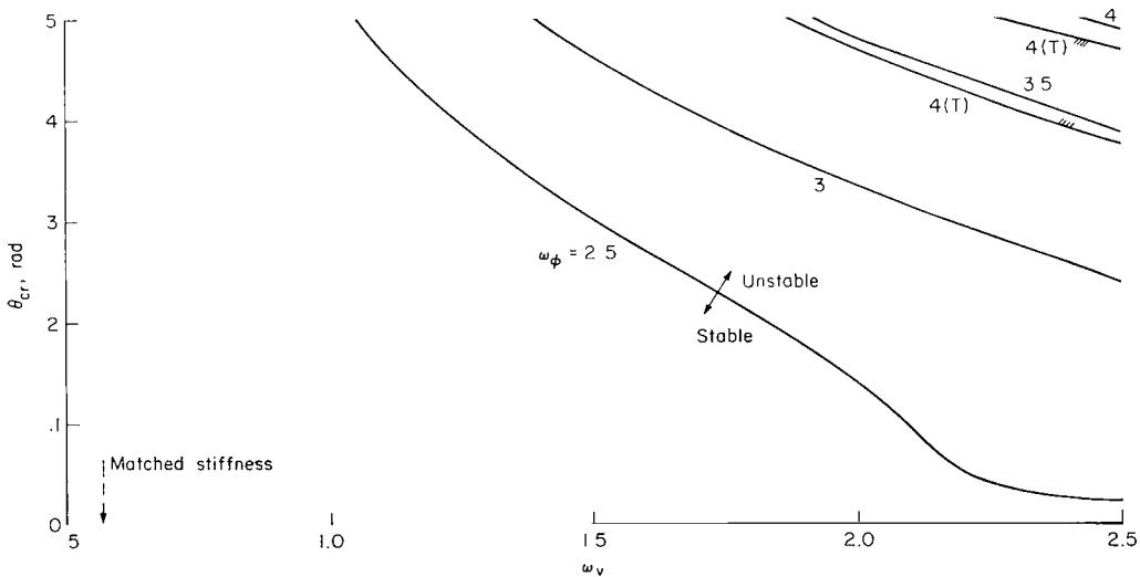
Figure 28.- The effect of torsion frequency on the stability boundaries,  $\theta_{cr}$  versus lead-lag frequency:  $\beta_{pc} = 0.0$  rad,  $\mathfrak{R} = 1.0$ .
