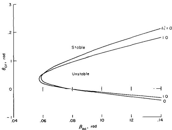
Figure 34.- The effect of  $R$  on the stability boundaries,  $\theta_{cr}$  versus precone angle:  $\omega_\phi = 2.5$ ,  $\omega_v = 0.7$ .
