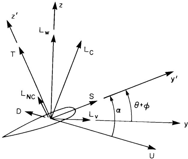
Figure 6.- Orientation of components of aerodynamic loading.
