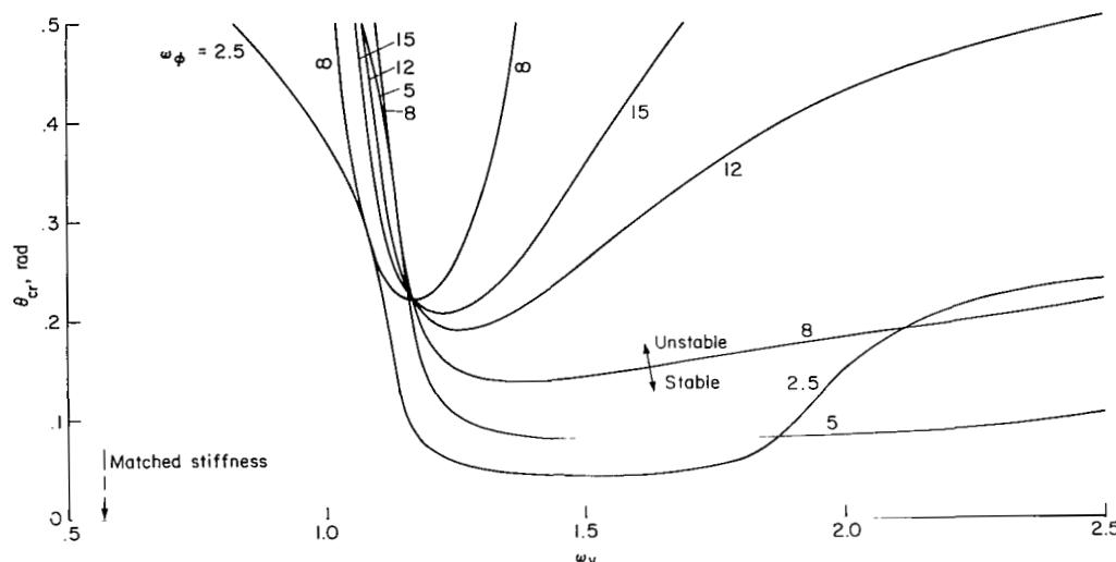
Figure 23.- The effect of torsion frequency on stability boundaries,  $\theta_{cr}$  versus lead-lag frequency:  $\beta_{pc} = 0.0$  rad,  $\Re = 0.0$ .
