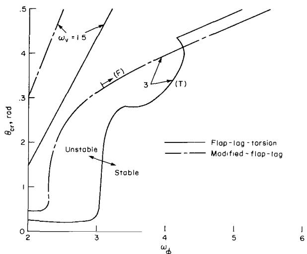
Figure 46.- The effect of approximations in the analysis on the stability boundaries,  $\theta_{cr}$  versus torsion frequency:  $\beta_{pc} = 0.0$  rad,  $R = 1.0$ .
