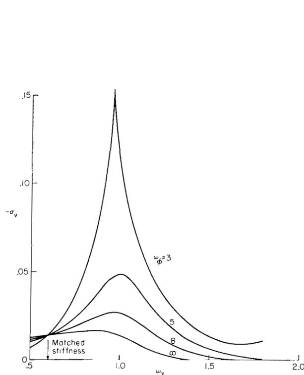
Figure 43.- The effect of torsion frequency on lead-lag modal damping versus lead-lag frequency:
