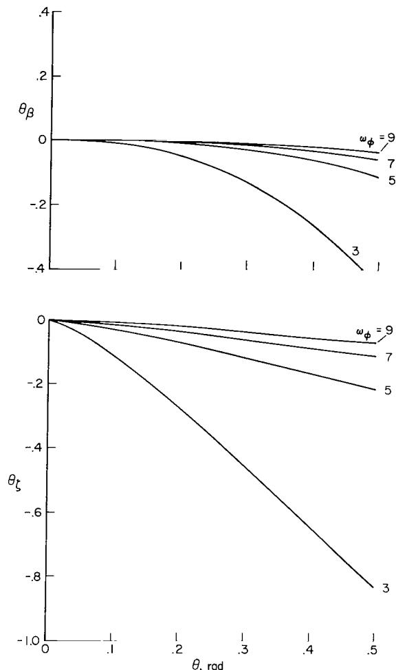
Figure 16.- Equivalent pitch-flap and pitch-lag coupling for a soft inplane rotor blade:  $\omega_v = 0.7$ ,  $\mathcal{R} = 1.0$ ,  $\beta_{pc} = 0.0$  rad.
