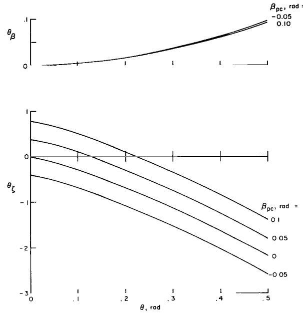
Figure 18.- Equivalent pitch-flap and pitch-lag coupling for a soft inplane rotor blade:  $\omega_v = 0.7$ ,  $\omega_\phi = 5.0$ ,  $\mathcal{R} = 0.0$ .
