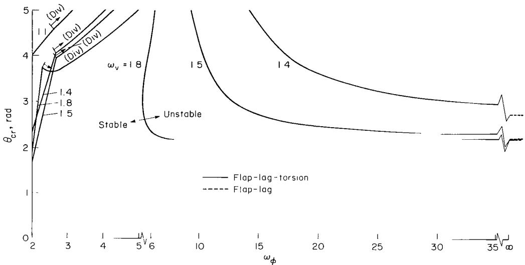
Figure 40.- The effect of lead-lag frequency on the stability boundaries,  $\theta_{cr}$  versus torsion frequency:  $\beta_{pc} = 0.0$  rad,  $\mathfrak{R} = 0.4$ .
