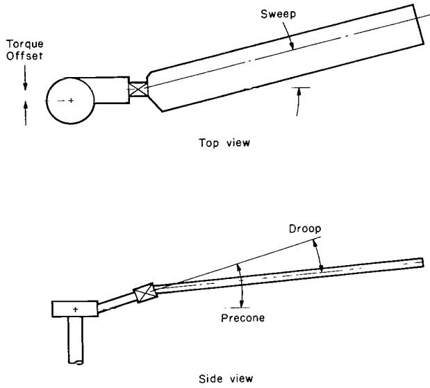
Figure 2.- Configuration parameters of a hingeless rotor blade (of these parameters only precone is considered in the present analysis).
