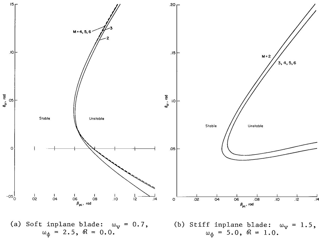
Figure 50.- Convergence of stability boundaries with respect to number of mode shapes for analysis using coupled rotating mode shapes; total number of mode shapes and degrees of freedom equals  $M$ . For each value of  $M$ , the coupled rotating mode shapes are derived from  $3N = 15$  uncoupled nonrotating mode shapes.
