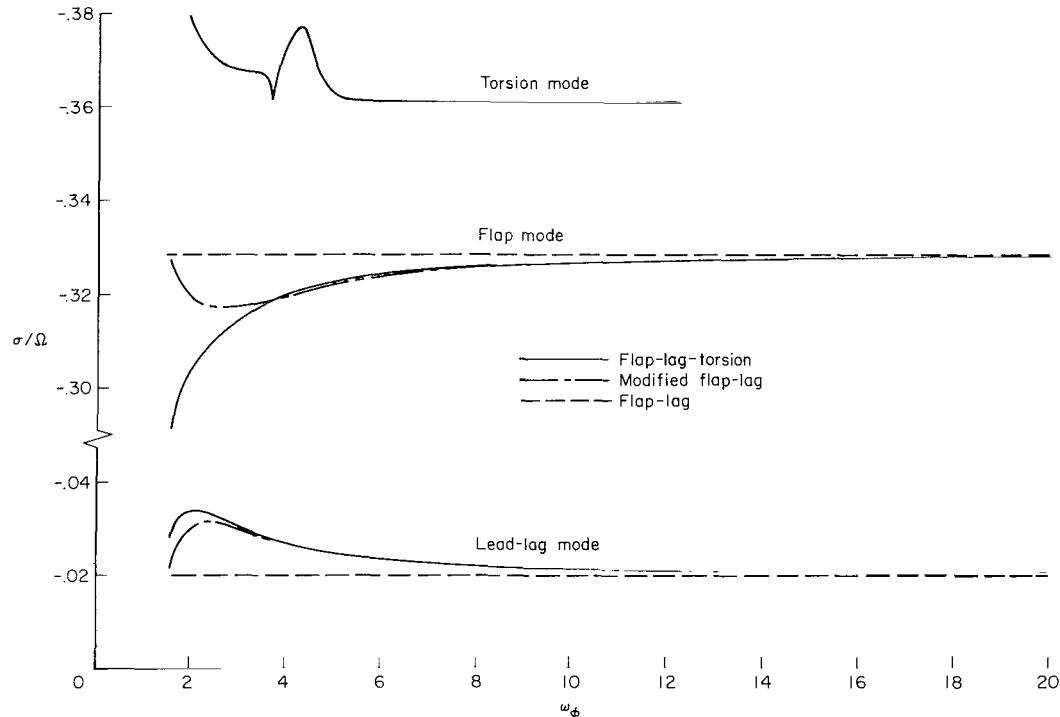
Figure 47.- The effect of approximations in the analysis on the flap, lead-lag, and torsion modal damping versus torsion frequency:  $\omega_v = 0.7$ ,  $\beta_{pc} = 0.0$  rad,  $\theta = 0.3$  rad,  $R = 1.0$ .
