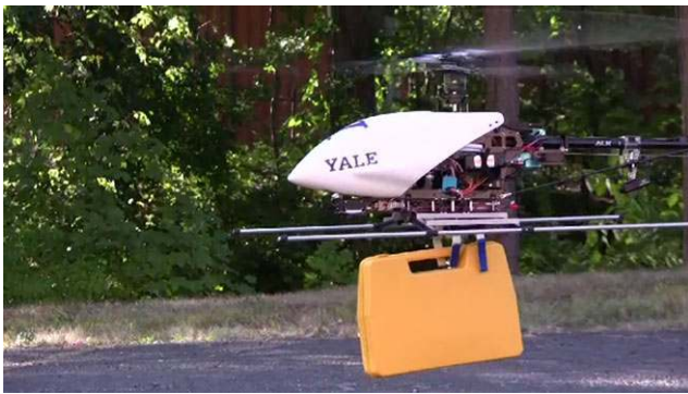
Fig. 1 Yale Aerial Manipulator carrying a 1.5 kg toolbox in hover
