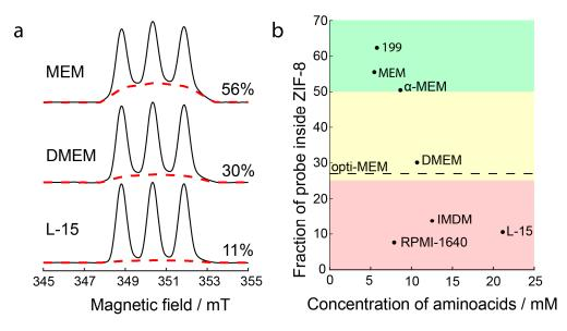
**Figure 3.** Dissolution of ZIF-8 in cell culture media. (a) First integrals of CW EPR spectra of R@ZIF-8 in culture media. Red dashed lines show the spectra obtained by simulation for a fraction of the probe inside ZIF-8. The numbers on the right demonstrate the weight of this fraction; (b) the fraction
