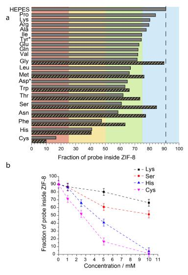
**Figure 4.** (a) Fraction of the probe inside ZIF-8 in R@ZIF-8 sample 5-fold diluted in HEPES (5 mM, pH = 7.4) containing 5 mM of individual amino acids. Hatching demonstrates samples with 10 mM MIM preliminary added to media. \* marks two amino acids with different concentrations—the highest we achieved considering the solubility of these amino acids in water (Table S2); (b)—Dependence of the probe inside ZIF-8 on amino acids concentration added.
