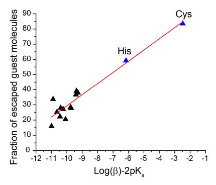
**Figure 5.** Correlation between a fraction of spin probes escaped from ZIF-8 and factor  $Log(\beta)$ -2pK<sub>a</sub>, being a combination of stability constant with zinc and pK<sub>a</sub> for amino acids (Table S3).
