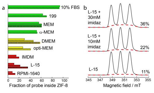
**Figure 6.** (a) Changes in fraction of probe inside ZIF-8, upon addition of different cell media (Table S2). Oblique hatching marks samples with addition of 10 mM MIM, vertical hatching—addition of 30 mM MIM; (b) first integrals of CW EPR spectra for R@ZIF-8 with addition of L-15 and MEM. Red dashed lines show the fraction of radicals remaining in ZIF-8; numbers on the right demonstrate the weight of this fraction.
