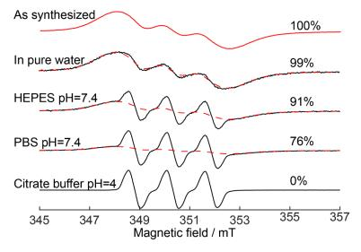
**Figure 2.** EPR spectra of initial suspension of R@ZIF-8 (as synthesized), R@ZIF-8 5-fold diluted in PBS (5 mM, pH = 7.4), HEPES (5 mM, pH = 7.4), and citrate buffer (0.1 M, pH = 4.0). Red dashed lines show the broad component in the spectra that corresponds to the probes located inside ZIF-8. The number on the right shows the amount of probe remaining inside ZIF-8 after dissolution.
