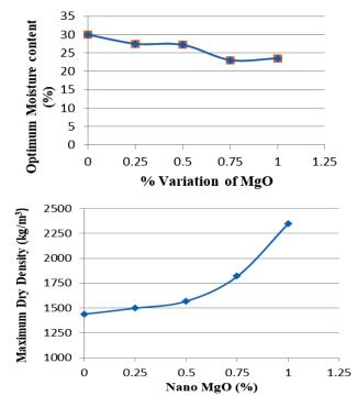
Figure 5: Outcomes of compaction study: a) OMC vs MgO, b) MDD vs MgO
