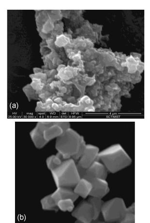
Figure 3: SEM images of annealed NC MgO attained by combustion technique: a) mag.  $30\ 000\ \times$ , b) mag.  $100\ 000\ \times$
