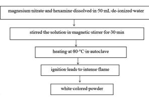
Figure 2: Flowchart for the synthesis of NC MgO
