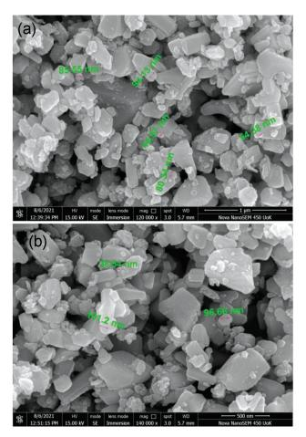
Figure 4: FE SEM images of nano ZnO powders: a) mag. 120 000 ×, b) mag. 140 000 ×
