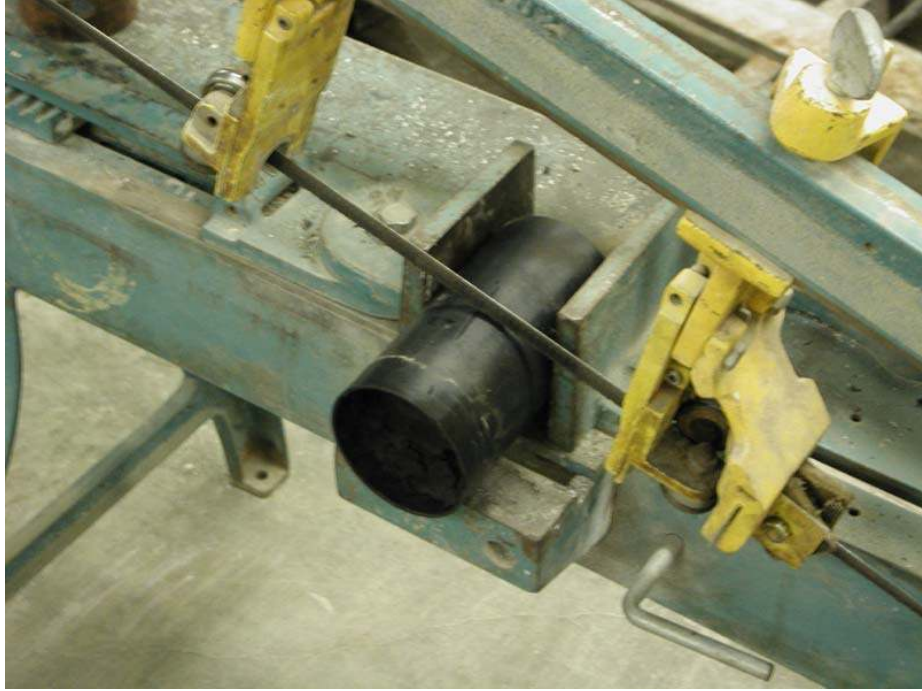
Figure 4.6: Cutting of plastic cylinder with Wells metal band saw for preparation of soil samples for CRS consolidation tests
