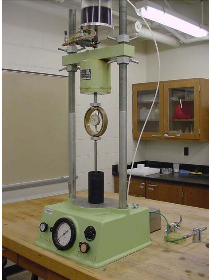
Figure 4.5: Stress control loading frame employed for preparation of treated MI and MII samples
