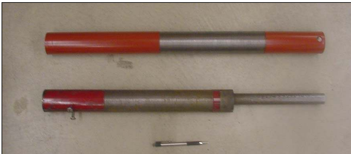
Figure 4.3: Original (D = 5.08 cm, above) and modified compaction hammer (D = 2.54 cm, below)
