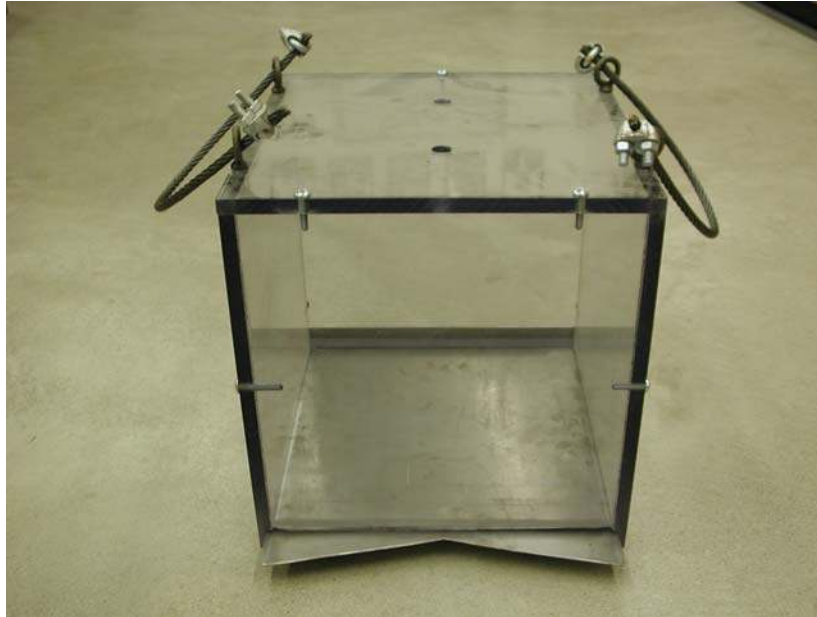
Figure 3.7: A 30cm x 30 cm x 30 cm block sampler made out of Lexan plates
