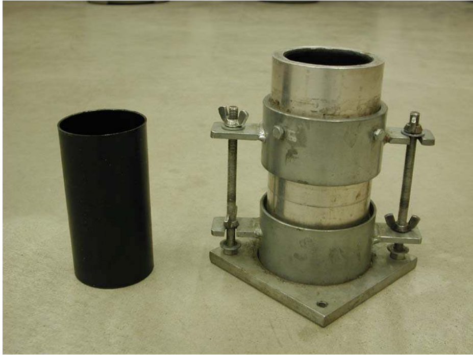
Figure 4.4: A plastic cylinder and modified compaction mold employed for compaction.
