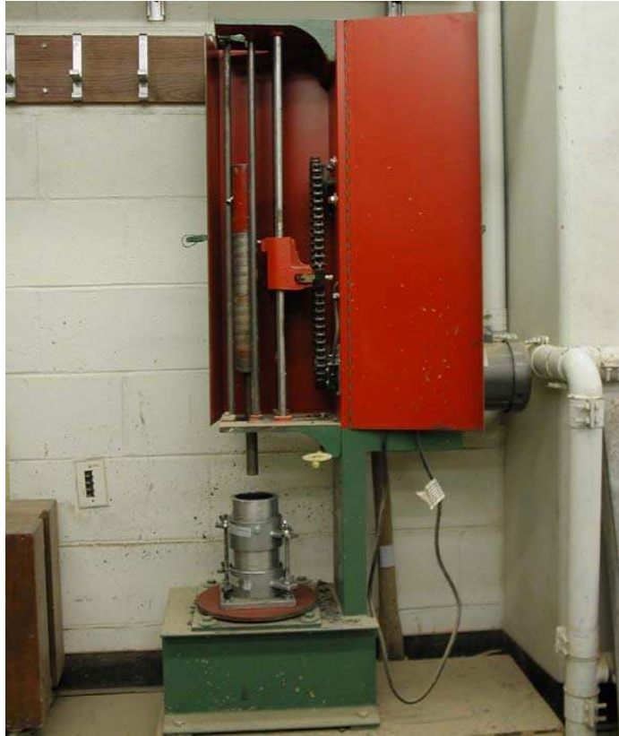
Figure 4.2: Modified mechanical proctor compactor employed for treated LR soil samples
