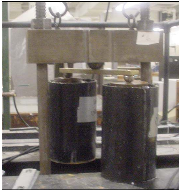
Figure 4.8: Specimen curing in consolidation frame under a surcharge of 96 kPa
