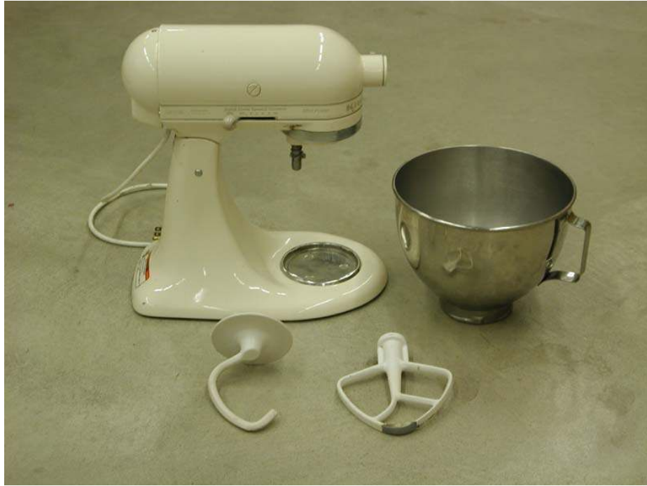
Figure 4.1: Mixer with two different mixing tools employed to prepare samples for CRS consolidation tests.
