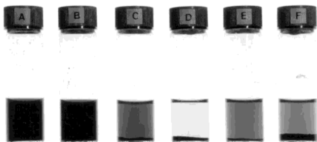
Figure 2. Vials containing aqueous dispersions of SWNT (0.05 wt %) after 3 months of incubation at room temperature: (A) 2 wt % GA; (B) 5 wt % GA; (C) 5 wt % SDS; (D) 15 wt % SDS; (E) 5 wt % CTAC; (F) 15 wt % CTAC. Note that a uniform dispersion (indicative of a single phase) is observed in A and B while in the other vials the carbon nanotubes coagulate at the bottom.
