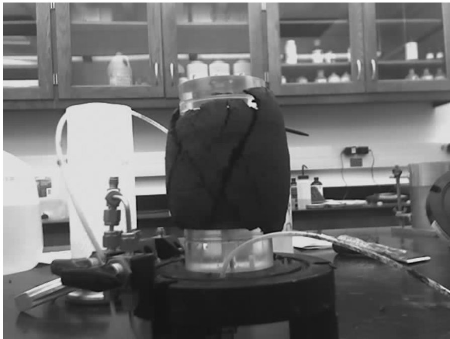
Figure 5-1: Typical Failure Mode for Organic Clay-MSW Ash Blends
