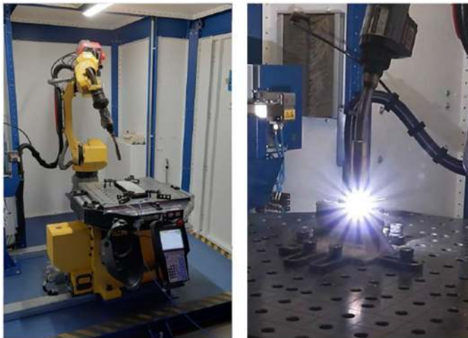
Fig. 18 Fanuc robot system using a TPS 500i MSG of Fronius as weld source, that was used to manufacture the compared workpieces. (left) Complete system, (right) welding head during printing process
