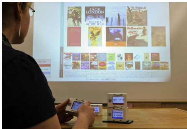
Figure 1: Stackables are small tangibles with display and two control wheels to adjust facet values. They can be combined to filter a complex faceted data set.
