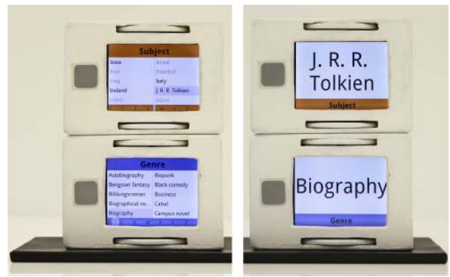
Figure 4: Two facet tokens in a stack. Left: The top showing the available values in black and the unavailable values in grey. Right: The same facet values after a period of inactivity.
