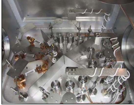
Fig. 3.9. Inside of the EvoVac chamber showing three metal sources, and eight organic sources.
