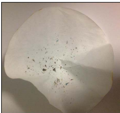
Fig. 4.25. Dried filter paper showing flakes of OLED constituents.
