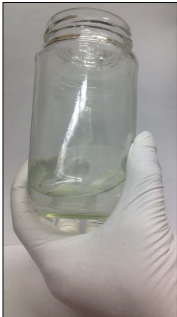
Fig. 4.26. The remaining solution after filtering. All macroscopic flakes of OLED constituents have been removed through the filtering process.
