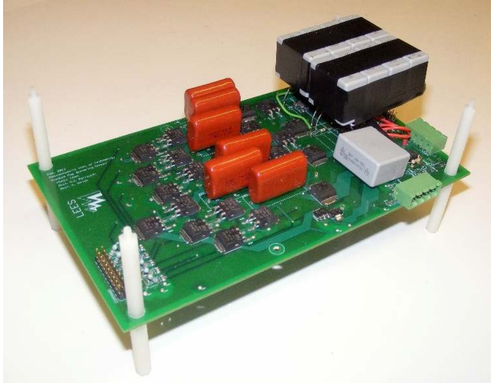
Figure 5-6: Prototyped bipolar 2-6 bipolar SSC energy buffer.
