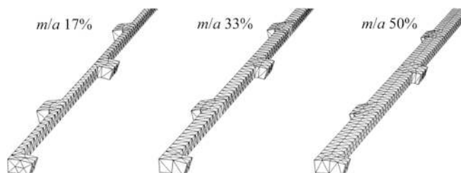
Fig. 3. CAD models of Palmaz-Schatz stents (SS stent) with different values of metal-to-artery ratio
