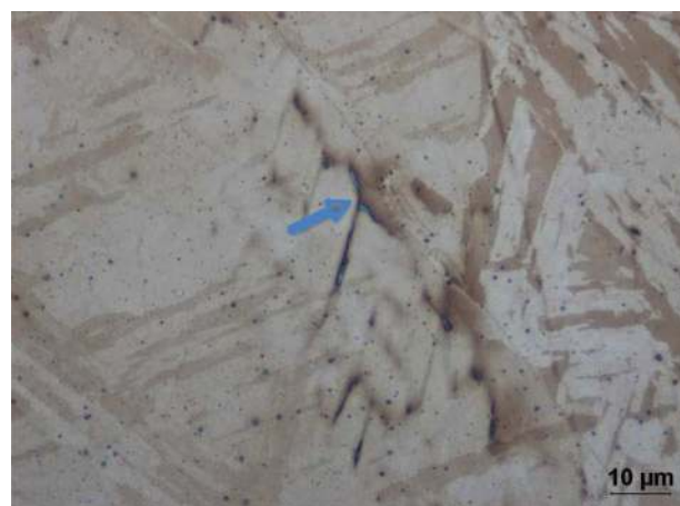
11 Alloy 2b multipass weld, etched using Kallings reagent: microstructure is predominantly martensitic with very small amount of \delta ferrite indicated by arrow
