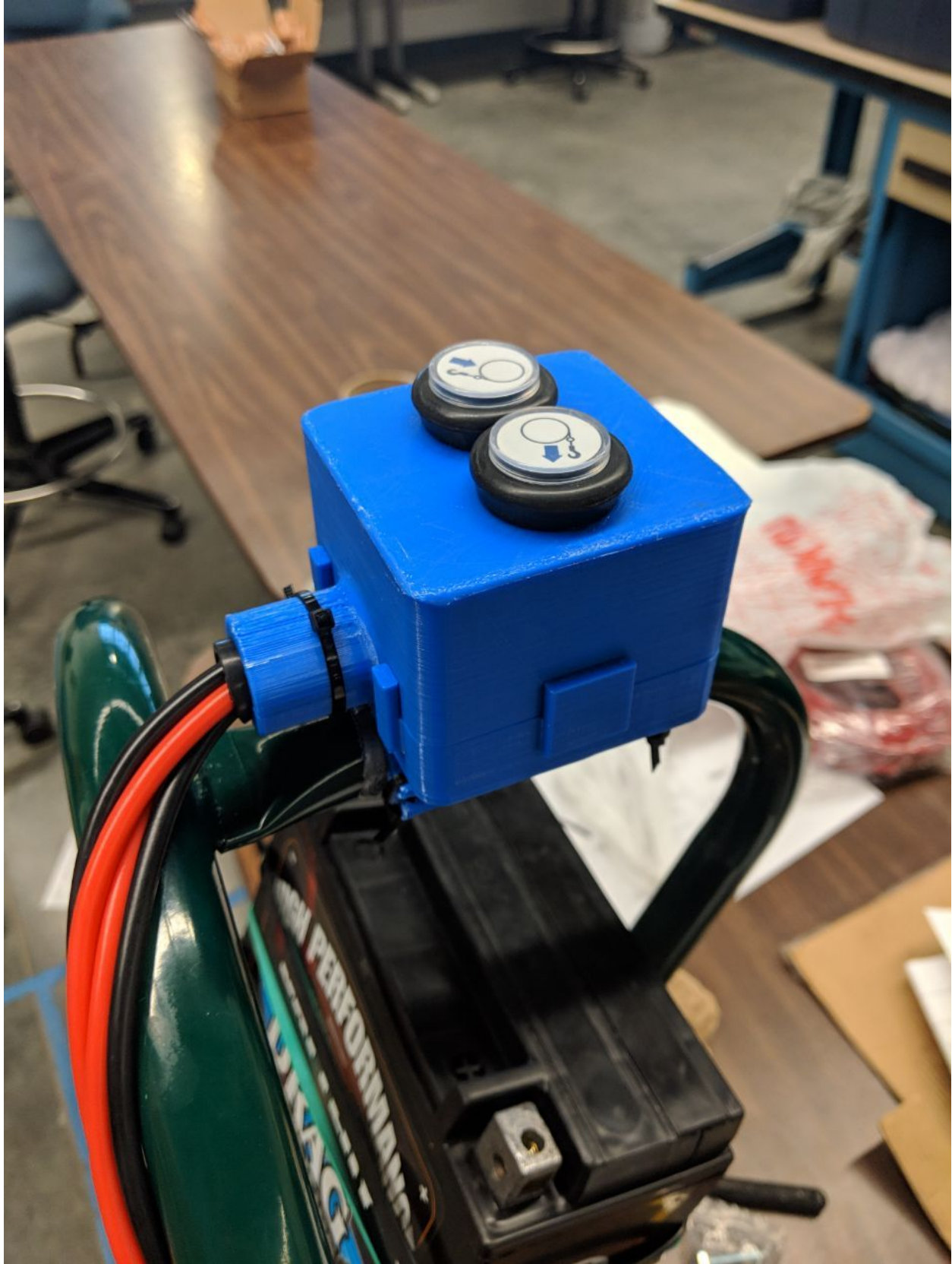
Photo of the finished and mounted 3D printed control housing
