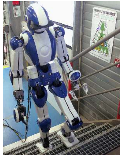
Fig. 1. HRP-4 humanoid climbing an industrial staircase at the Airbus factory in Saint-Nazaire, France. Step height is 18.5 cm. The experiment was reproduced time and again over the course of two weeks spent on-site, and deemed robust enough to let the robot climb without safety ropes.
