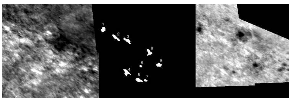
Figure 8 ROI B - Anomaly detection results; Left: mosaic IR at 09:59; Right: mosaic IR at 01:46; Middle: detected anomalies.
