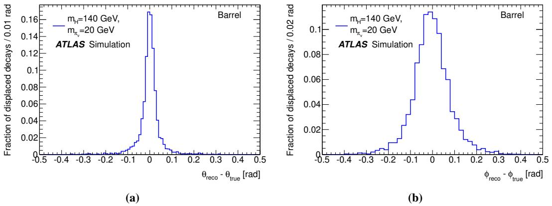
**Figure 11.** Distributions of the flight direction residuals in the (a)  $\theta$  and (b)  $\phi$  directions. Both plots show the MC mass point  $m_H = 140 \text{ GeV}$ ,  $m_{\pi_v} = 20 \text{ GeV}$ . Similar results are found using the other MC samples.
