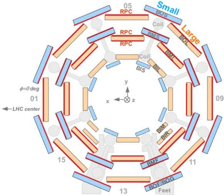
**Figure 2.** Cross-sectional view of the barrel muon spectrometer perpendicular to the beam axis (non-bending plane). The MDT chambers in the small sectors are shown in light blue, the MDT chambers in the large sectors are shown in orange and the RPC chambers in red. The eight coils are also visible.
