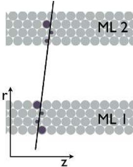
**Figure 3.** Portion of a muon spectrometer barrel chamber (BIL) with two four-layer multilayers. The drift circles are shown in dark gray and the charged particle trajectory is shown as the black line. The spacing between the two multilayers is 170 mm.
