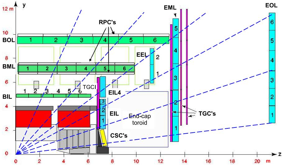
**Figure 1.** Cross-sectional view of ATLAS in the  $r$ - $z$  projection at  $\phi = \pi/2$ , from ref. [1]. The barrel MDT chambers are shown in green, the endcap MDT chambers are blue. In the barrel (endcaps), the RPC (TGC) chambers are shown outlined in black (solid purple).
