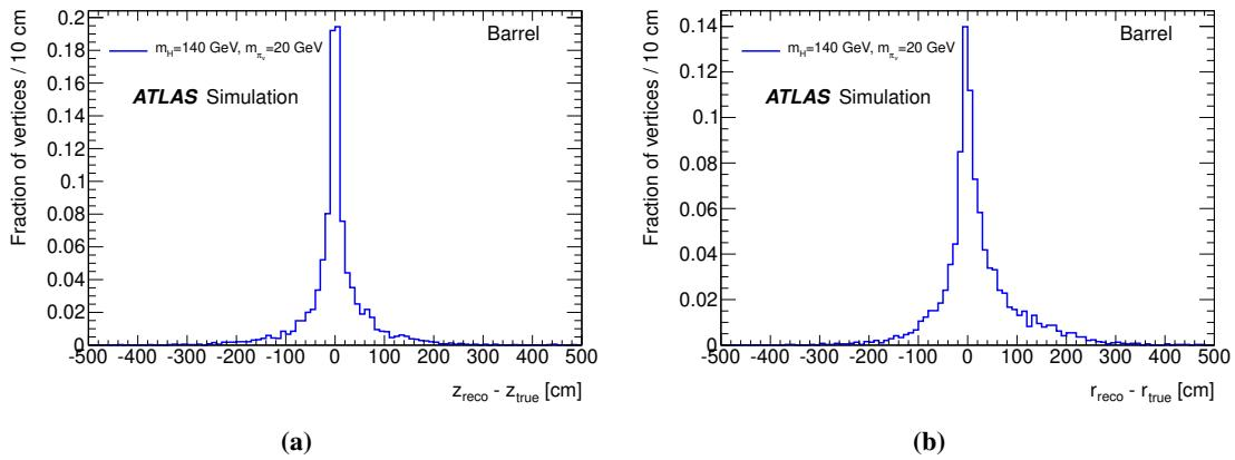
**Figure 13.** Distributions of the vertex-reconstruction residuals in the (a)  $z$  coordinate and (b)  $r$  coordinate for decays in the barrel MS. Both plots show the MC mass point  $m_H = 140 \text{ GeV}$ ,  $m_{\pi_v} = 20 \text{ GeV}$ . Similar results are found using the other MC samples.
