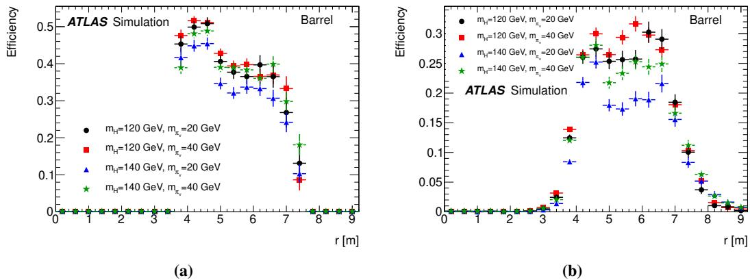
**Figure 17.** Efficiency for reconstructing a vertex for  $\pi_v$  decays in the barrel muon spectrometer as a function of the radial decay position of the  $\pi_v$  for (a)  $\pi_v$  decays that satisfy the Muon RoI Cluster trigger and (b)  $\pi_v$  decays that do not satisfy the Muon RoI Cluster trigger.
