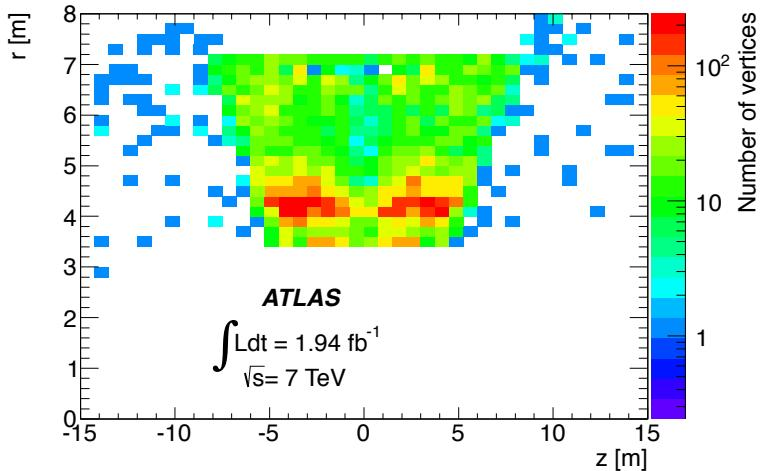
**Figure 20.** Distribution of the position, in  $(r,z)$ , of all good vertices in the fiducial volume of the muon spectrometer in events that passed the barrel Muon RoI Cluster trigger from  $1.94 \text{ fb}^{-1}$  of  $7 \text{ TeV}$   $pp$  collision data.
