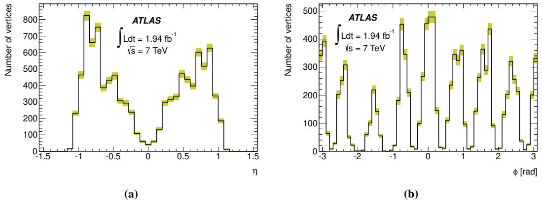
**Figure 19.** Distribution of the (a)  $\eta$  and (b)  $\phi$  position of the good vertices reconstructed in the data events that pass the Muon RoI Cluster trigger. The statistical uncertainty on the data points is represented by the yellow bands. The effect of extra material present in the feet is visible as a relative decrease in the number of vertices reconstructed in the region between  $\phi = -1$  and  $\phi = -2$ .
