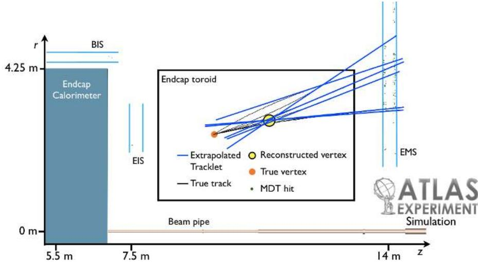
**Figure 15.** Diagram illustrating the reconstruction technique employed in the endcap muon spectrometer. The display shows the simulated decay of a  $\pi_v$  from the MC mass point  $m_H = 140$  GeV,  $m_{\pi_v} = 20$  GeV.
