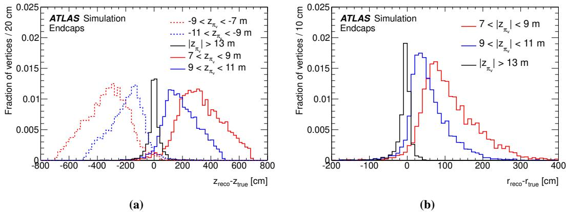
**Figure 14.** Distributions of the vertex-reconstruction residuals in the (a)  $z$  coordinate and (b)  $r$  coordinate for decays in the endcap MS for different ranges of  $z_{\pi_v}$ . Both plots show the MC mass point  $m_H = 140$  GeV,  $m_{\pi_v} = 20$  GeV. Similar results are found using the other MC samples.
