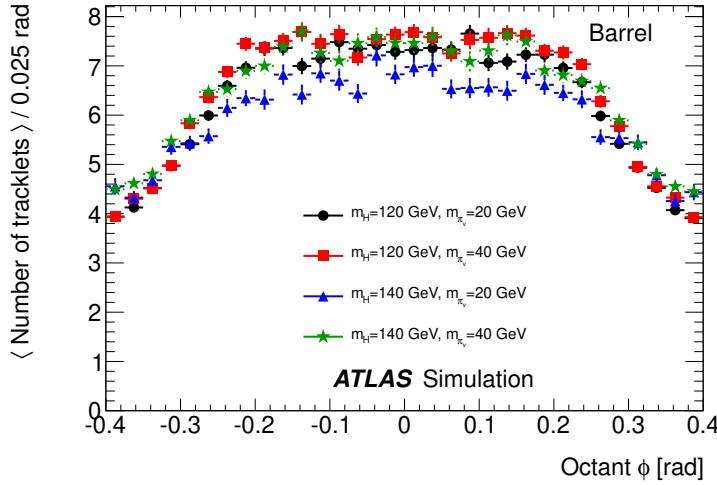
**Figure 9.** The average number of tracklets with a charge and momentum measurement reconstructed as a function of the position, in  $\phi$ , of the displaced decay, for decays occurring in the barrel MS. All sectors have been projected such that the centre of a large sector corresponds to  $\phi = 0$  and the centre of a small sector corresponds to  $\phi = \pm\pi/8$ .
