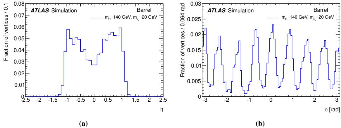
**Figure 16.** Distribution of the (a)  $\eta$  and (b)  $\phi$  positions of the good vertices in the barrel muon spectrometer for the Monte Carlo signal samples. Both plots show the MC mass point  $m_H = 140 \text{ GeV}$ ,  $m_{\pi_v} = 20 \text{ GeV}$ . Similar results are found using the other MC samples.
