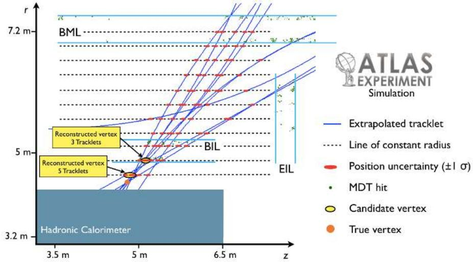
**Figure 12.** Diagram illustrating the reconstruction technique employed in the barrel muon spectrometer. The display shows the simulated decay of a  $\pi_v$  from the MC mass point  $m_H = 140 \text{ GeV}$ ,  $m_{\pi_v} = 20 \text{ GeV}$ .
