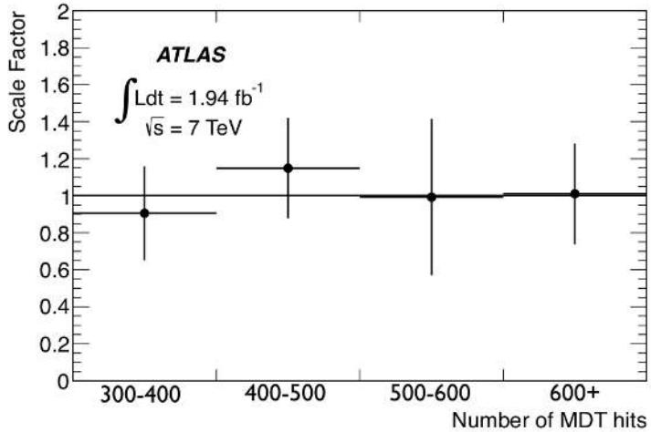
**Figure 21.** The scale factor calculated by dividing the fraction of punch-through jets in data that have a good MS barrel vertex by the fraction in Monte Carlo simulation. The scale factor is calculated as a function of the number of MDT hits inside a cone of size  $\Delta R = 0.6$ , centred around the jet axis.
