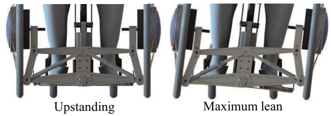
Fig. 8. Link mechanism for leaning
