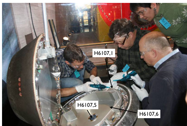
Fig. 7. Sampling of the sample return capsule backshell at the Smithsonian Air and Space Museum, showing the locations of 3 of the 5 chips.
