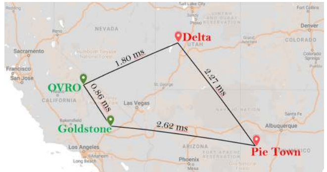
FIG. 6.— Map of STARE2 stations with light travel time delays between the baselines. The OVRO and Goldstone sites in green are operational, while the Delta and Pie Town sites in red are options for additional stations.
