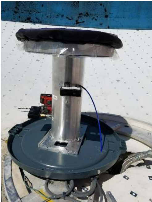
FIG. 3.— The choke-ring feed located at OVRO. It lies in a 6 m dish which is used as a horizon shield. The 6 m dish blocks up to 25^\circ above the horizon. The 6 m dish blocks up to 25^\circ above the horizon. 191 Mpc is \sim 33\% .
