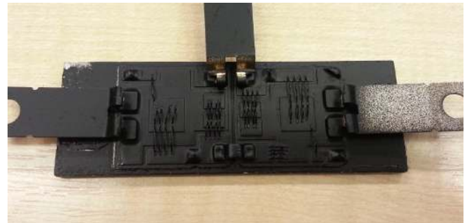
Fig. 6 To overcome the emissivity variation, IGBT sample covered with black matt paint prepared for thermal recording by IR camera.
