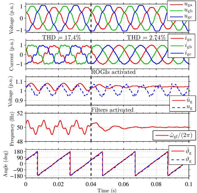
Fig. 16. Measured three-phase grid voltages (first), three-phase grid currents (second), the estimated and actual grid-voltage magnitudes (third), estimated angular frequency  $\hat{\omega}_{gf}$  (fourth), and estimated and actual grid-voltage angles (fifth), when the grid voltages are distorted and unbalanced. After  $t = 0.04$  s, generalized integrators in the current controller and the notch filters in the adaptation loops and DC-voltage control are activated.
