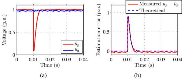
Fig. 11. Experimental results when the disturbance impulse of  $-0.9$  p.u. is applied into the estimated grid-voltage magnitude: (a) estimated and actual magnitudes; (b) measured magnitude-estimation error and corresponding theoretical response from (29).
