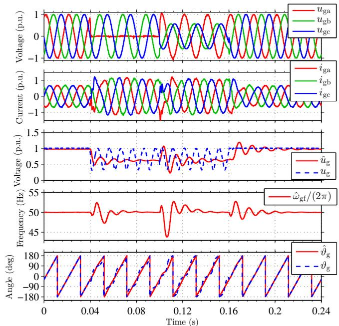
Fig. 17. Measured three-phase grid voltages (first), three-phase grid currents (second), the estimated and actual grid-voltage magnitudes (third), estimated angular frequency  $\hat{\omega}_{gf}$  (fourth), and estimated and actual grid-voltage angles (fifth), when unbalanced grid-voltage dips are applied.
