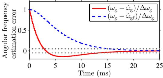
Fig. 6. Estimation-error responses when a step change  $\Delta \omega_g$  is applied in  $\omega_g$ : (solid line) angular-frequency estimate  $\hat{\omega}_g$ ; (dashed line) angular-frequency estimate  $\hat{\omega}_{gf}$ . The tuning parameters of the adaptation loop are:  $\omega_\omega = 2\pi \cdot 50$  rad/s and  $\zeta_\omega = 1$ . The 5%- settling limits are marked with dotted lines.
