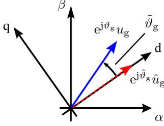
Fig. 3. Orientation of the estimated grid-voltage reference frame.
