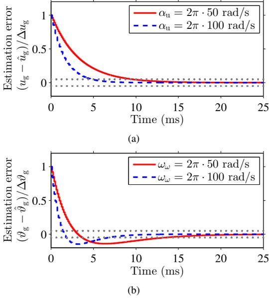
Fig. 5. Estimation-error responses: (a) step change  $\Delta u_g$  is applied in the grid-voltage magnitude  $u_g$  at  $t = 0$  in (24); (b) step change  $\Delta \vartheta_g$  is applied in the angle  $\vartheta_g$  at  $t = 0$  in (26). The tuning parameters of the adaptation loops are varied according to the legends. The damping ratio is  $\zeta_\omega = 1$ . The 5%- settling limits are marked with dotted lines.
