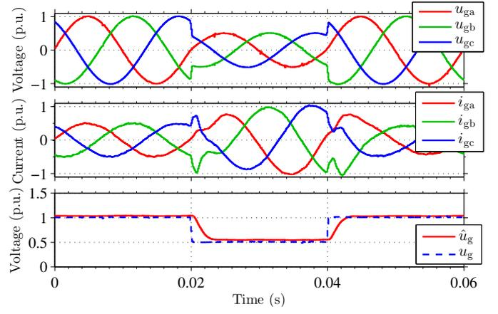
Fig. 13. Measured grid voltages  $u_{ga}$ ,  $u_{gb}$ , and  $u_{gc}$  (above), grid currents  $i_{ga}$ ,  $i_{gb}$ , and  $i_{gc}$  (middle), and the estimated and actual grid-voltage magnitudes (below), when a grid-voltage dip is applied.
