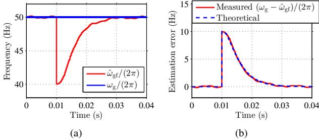
Fig. 12. Experimental results when the disturbance impulse of  $-10$  Hz is applied into the estimated grid-voltage frequency: (a) estimated and actual frequencies; (b) measured frequency-estimation error and corresponding theoretical response from (29).
