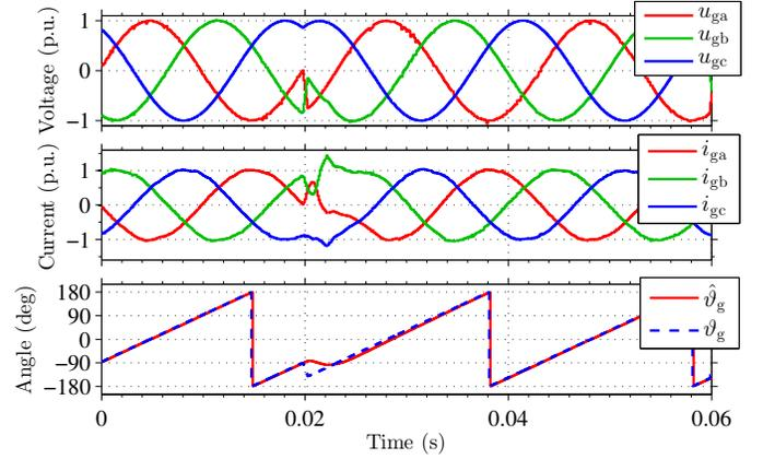
Fig. 14. Measured grid voltages  $u_{ga}$ ,  $u_{gb}$ , and  $u_{gc}$  (above), grid currents  $i_{ga}$ ,  $i_{gb}$ , and  $i_{gc}$  (middle), and the estimated and actual grid-voltage angles (below), when a grid-voltage angle is changing rapidly  $-60^\circ$ .
