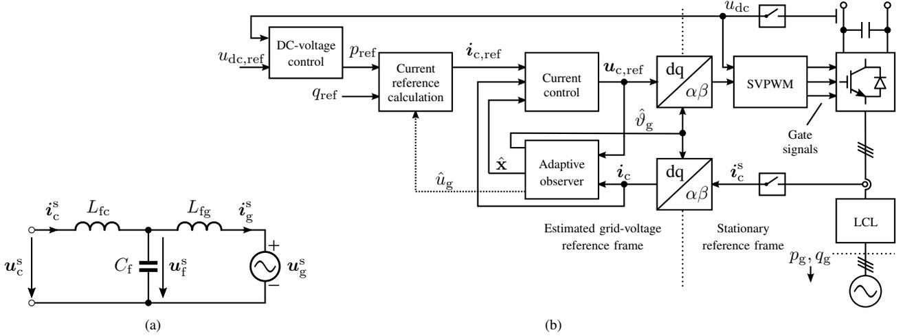
Fig. 1. (a) Space-vector circuit model of the grid-connected LCL filter in stationary coordinates (marked with the superscript s). (b) Grid-voltage sensorless control system. The angle  $\omega_g T_s$  caused by the computational delay is compensated for in the  $dq \rightarrow \alpha\beta$  transformation (not explicitly shown in the figure).
