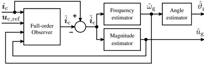
Fig. 2. Internal structure of the adaptive observer.
