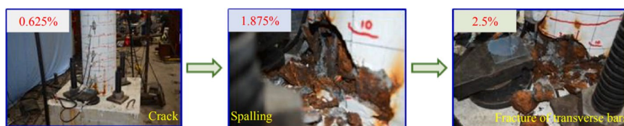
Fig. 22 Damage process at 10% corrosion level
