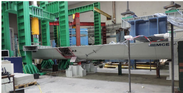
Fig. 12 Steel box girder with curved stiffened plates at the bottom
