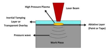
Figure 2. Schematic representation of the laser shock peening process [30].
