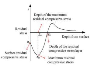
Figure 6. Evaluation of shot peening performance based on distribution of residual stress on target [17].
