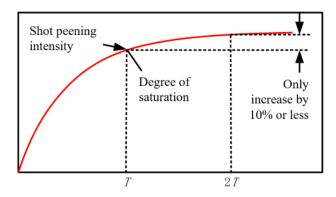
Figure 5. Saturation state curve [73].
