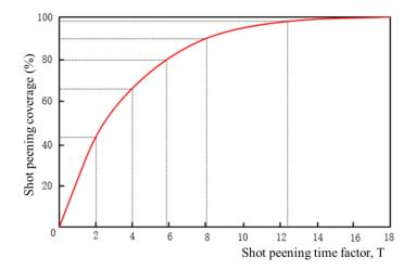
**Figure 10.** Experimental results of the relationship between shot peening coverage and shot peening time factor [84].
