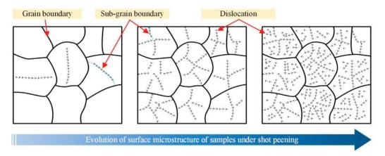
Figure 8. Schematic representation of microstructure evolution under shot peening [78].
