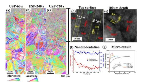
**Figure 9.** The microstructure refinement and mechanical strengthening of dual-phase high entropy alloy during ultrasonic shot peening [80].
