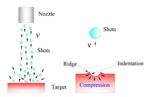
gained widespread use in industries such as aerospace and automotive, due to its ability to increase the resistance of components to fatigue failure and wear failure.
