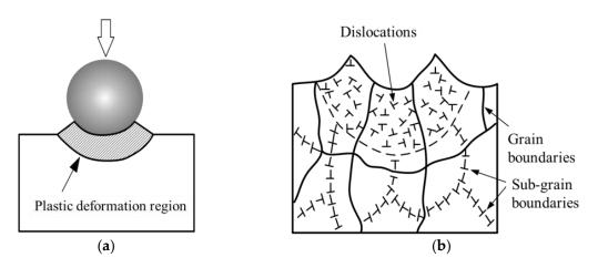
**Figure 7.** (a) Plastic deformation caused by ball impacting the workpiece surface, (b) microstructure of workpiece after ball impacting [75].
