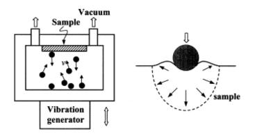
Figure 3. Schematic representation of the ultrasonic shot peening process [39].
