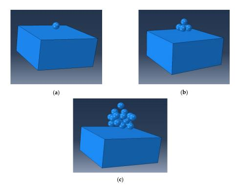
**Figure 4.** Numerical model of the shot peening process: (a) single shot, (b) regular array shot, (c) random shot.
