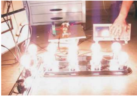
(b) 88% efficiency is achieved, transmitting 1kW of power [57]. Reproduced with permission, ©SPIE 2008. All rights reserved
