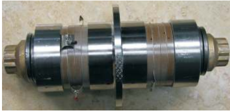
(a) 1kW power transfer through metal wall [56]. Reproduced with author permission, ©NASA 2008. All rights reserved
