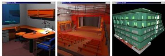
Figure 1: Interactive ray tracing: The office, conference and Soda Hall models contain roughly 40k, 680k, and 8 million triangles, respectively. Using a software ray tracing implementation running on a single PC (Dual Pentium-III, 800 MHz, 256MB) at a resolution of 512 2 pixels, these scenes render at roughly 3.6, 3.2, and 1.6 frames per second.
