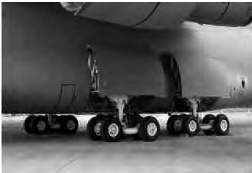
Fig. 13. Undercarriages of B52 and C-5 Galaxy transport aircraft
