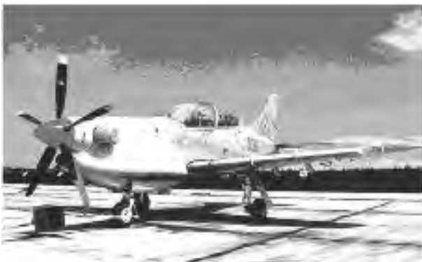
Fig. 3. PZL-130 TC Orlik military primary trainer – airplane with turbo engine and telescopic nose landing gear and trailing arm main landing gear both retractable (take-off mass 2700 kg)
