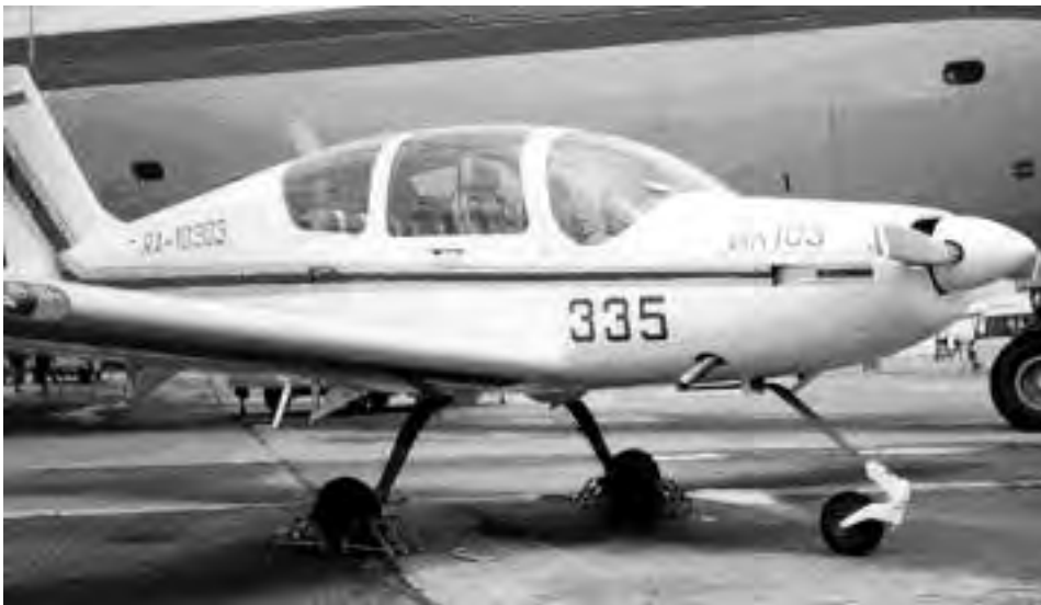
Fig. 18. Spring type non-retractable landing gear
