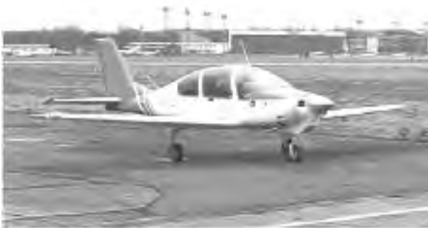
Fig. 1. I-23 Executive airplane with piston engine and cantilever retractable landing gear – nose and main (take-off mass 1150 kg)
