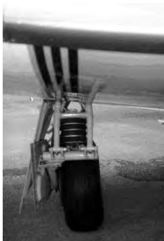
Fig. 19. Retractable landing gear with spring rubber elements
