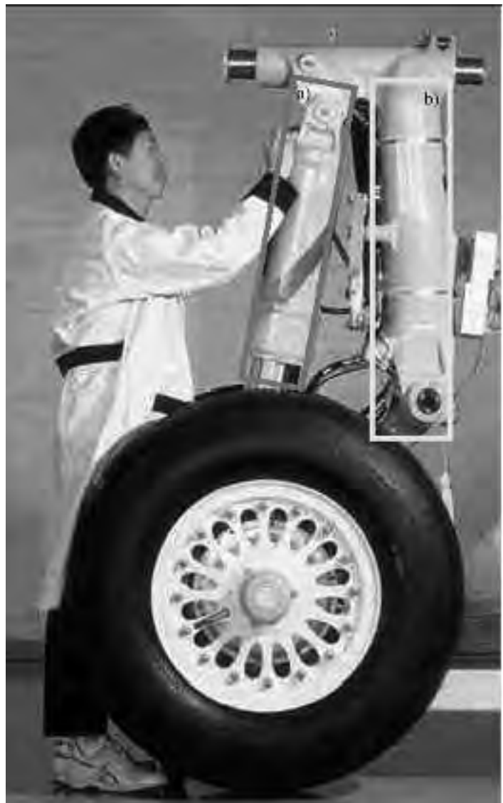
Fig. 17. Bombardier Global Express main landing gear a) shock absorber b) main strut
