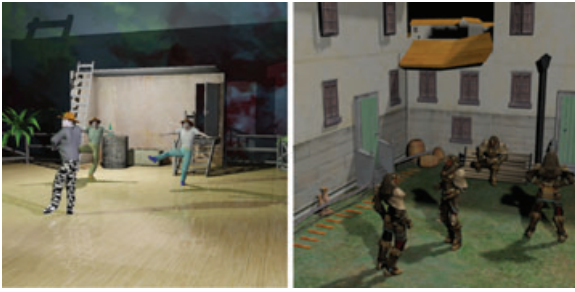
Figure 1: Left: using Shevtsov et al.'s technique, this scene with 63k static and 171k animated triangles can be ray traced with 7.2 fps at 1024^2 pixels on a four core 3 GHz Intel Core 2 Duo including shadows from two point lights [SSK07]. Right: using Hunt et al.'s technique [HMF07], the kd-tree acceleration structure for this view of this scene with 541023 quads (of which 9392 are visible) is lazily built in 0.12 seconds on a single core of a 2.67 GHz Intel Core 2 Duo.
