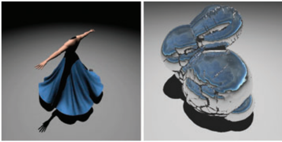
Figure 5: Two screenshots from Lauterbach et al.'s BVH based ray tracing system. Left: one frame from a 40k triangle dress simulation animation, running at 13 frames per second ( 512 \times 512 pixels, one point light) on a dual 2.8 GHz Pentium IV PC. Right: a fracturing bunny including shadows and reflections, running at an average of six frames per second on same hardware.
