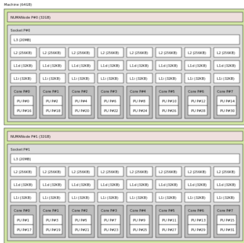
Figure 4: The output of lstopo , a tool provided by hwloc [BCOM*10] to visualize hardware topology. The memory hierarchy is shown as a hierarchical space-filling layout, with larger resources at the root and smaller caches and processors at the leaves.
