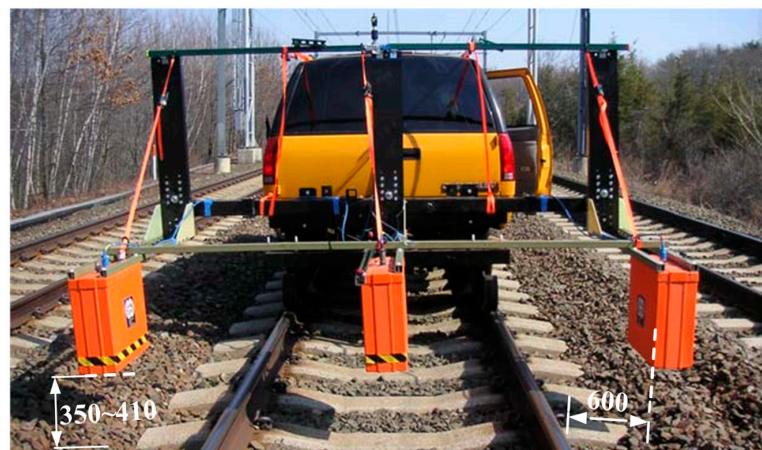
(a) GPR system with carrier (a van)
