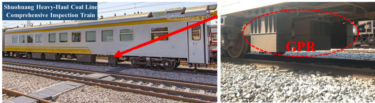
Figure 16. Integrated inspection vehicle with GPR system.
