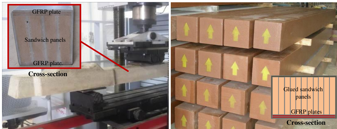
(a) Timber replacement sleeper
