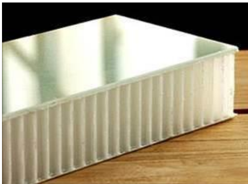
(c) Honeycomb core
