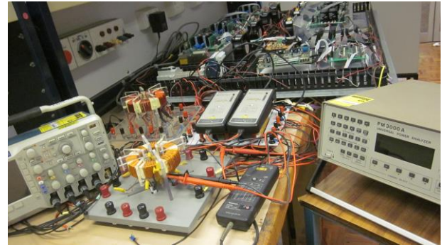
Fig. 5. A photograph of the test platform to measure specific core loss of high-frequency transformer [51].
