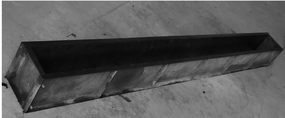
Fig. 4 Form work of the test specimens
