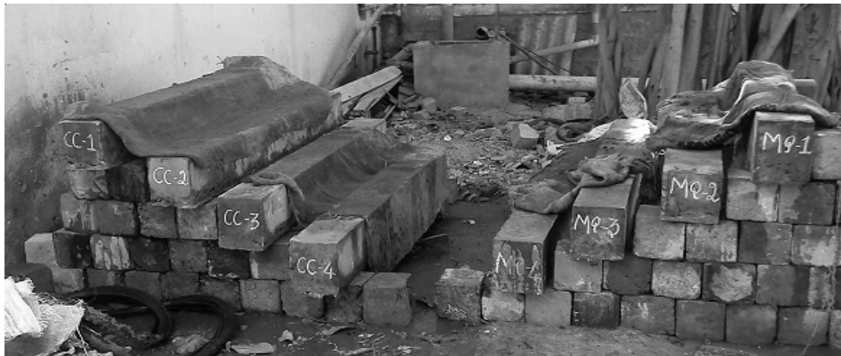
Fig. 5 Test specimens Flexure beam under Curing
