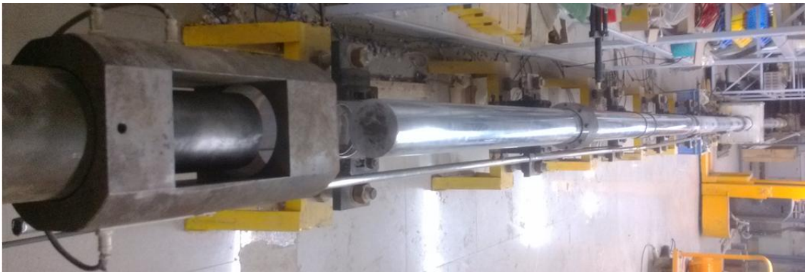
(b) Picture of SHPB equipment
