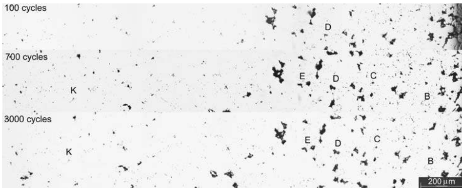
Fig.12. Microcrack initiation and development in the first 3000 cycles. Note that (i) microcrack D initiation within the first 100 cycles,(ii) at 700 cycles: growth of D and 4 new microcracks B, C, E nucleated at N=600 and K nucleated at N=200 ,(iii) growth of microcracks B, D, E and K between 700 and 3000 cycles, whilst C was dormant.
