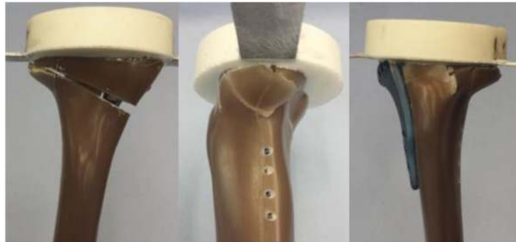
Fig. 5 Fracture of the contralateral cortical bone during the fatigue testing: The specimens failed by fracture of the contralateral cortical bone, similar to the static tests
