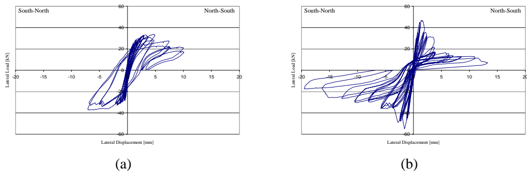
Figure 11 Lateral forces vs. relative top wall displacement for (a) S2-REFE-ST, and (b) S2-WRAP-G-F-ST
