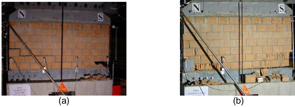
Figure 5 Specimens (a) S2-REFE-ST and (b) S2-WRAP-G-F-ST (unreinforced face) at the test end
