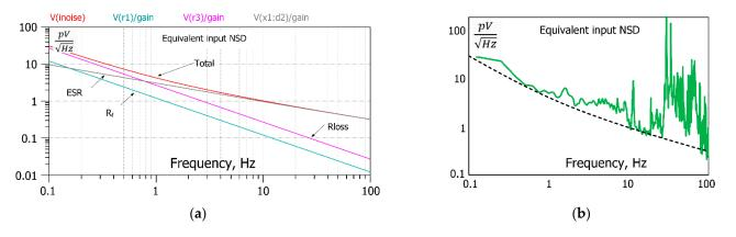
**Figure 16.** Simulated equivalent input magnetic noise spectral density (**a**) total equivalent input noise spectral density and contribution of dielectric noise, DC resistance noise, and feedback resistor. (**b**) Simulated equivalent input noise spectrum compared with equivalent input noise spectrum measured in [29]. The data is adapted with permission form ref. [29], 2011, John Wiley and Sons.
