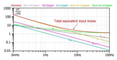
**Figure 15.** The equivalent input noise and the equivalent input noise components due to each noise source. The dominant noise source  $i_n$  is the equivalent current noise source of amplifier U1. The equivalent voltage noise units V/Hz<sup>1/2</sup> correspond to magnetic field noise units T/Hz<sup>1/2</sup>.
