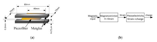
**Figure 2.** An example of a magnetoelectric sensor was proposed in [29]. (**a**) Mechanical topology and dimensions. All the layers are bonded mechanically with epoxy resin. (**b**) Block diagram of multi-domain signal conversion starting from the magnetic domain to the mechanical domain and then to the electrical domain.
