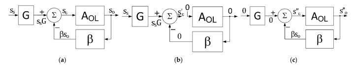
**Figure 4.** The block diagram of the system with feedback. (a) General form, where  $A_{ol}$  is an open loop gain of the amplifier, *G* is a constant gain,  $\beta$  is a feedback gain, and  $\Sigma$  is a summing unit. The signals are:  $s_s$  is a source signal,  $s_o$  is an output signal, and  $s_\varepsilon$  is an error signal. (b) The circuit with the disabled error signal  $s_\varepsilon$  and nonzero source signal  $s_s$ . (c) The circuit with the disabled source signal  $s_o$ .
