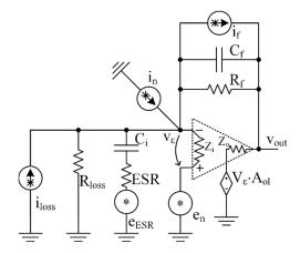
**Figure 11.** A map of noise sources. The  $i_{loss}$  is the current noise corresponding to the thermal noise of the leakage resistance  $R_{loss}$  and the  $e_{ESR}$  is the ESR voltage noise source. The  $e_n$  and  $i_n$  are correspondingly the voltage and the current equivalent input noise sources of the opamp, and  $i_f$  is the current noise source of the feedback resistor  $R_f$ . All the resistors and opamp are noiseless.
