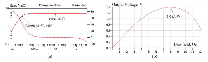
**Figure 13.** The frequency sweep of the model signals. (a) The solid line is a small signal gain (left axis), and the dashed line is the phase (right axis) of the transfer function of the charge amplifier in the frequency range of interest. (b) Output voltage at an input signal of 10 nT vs. the bias magnetic field.
