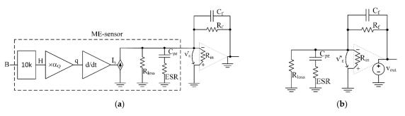
**Figure 6.** Simplified schemes for defining the components of a block diagram of a feedback system: (a) the error signal  $v'_{\epsilon}$  is suppressed while the input signal *B* is nonzero and (b) the input signal *B* is suppressed while the output signal  $v_{out}$  is nonzero.
