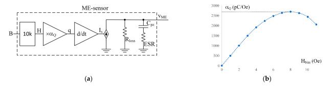
**Figure 3.** The equivalent diagram of the ME sensor is shown in (**a**). The charge *q* is proportional to the field *H* with the coefficient  $\alpha_Q$ . The  $\alpha_Q$  vs.  $H_{bias}$  is shown in (**b**). The data for the plot adapted with permission from ref. [29]. 2011, John Wiley and Sons. An input signal is a magnetic flux *B* [T] corresponding to a magnetic field *H*[Oe] in the air with a factor of 10 k.
