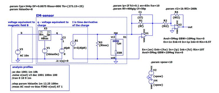
**Figure 12.** Scheme for simulating an ME sensor with a two-stage charge amplifier implemented in the LTSPICE environment. The hierarchical blocks circuitry X1 and X2 are shown in Figures 9 and 10. Opamps U1 and U2 use a modified built-in "universalopamp" model. All values of each element are provided in the schematic as global parameters under directive **param**. Each circuit element references a specific parameter in curly brackets. All the parameters are described in Table 4.
