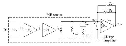
**Figure 5.** ME-sensor equivalent scheme (Figure 3) with charge amplifier circuitry. The charge amplifier consists of an opamp with open-loop gain  $A_{ol}$ , input impedance  $R_{in}$ , and the feedback elements  $C_f$  and  $R_f$  that form the gain and bandwidth. An output impedance of the opamp is negligible compared to a feedback resistor at low frequencies.
