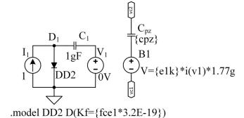
**Figure 9.** A hierarchical block of the capacitance and the *ESR* thermal noise of the piezoelectric material as it looks in LTSpice, where vc1 and vc2 are capacitor terminals, cpz is a parameter of the capacitance of the piezoceramic element, *boltz* is a PSPICE built in Boltzmann's constant, *Tk* is a temperature in kelvin, *fce1* is the  $f_{C_{ESR}}$ , and *e1k* is the  $e_{n_{ESR}}$ .
