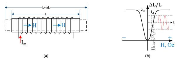
**Figure 1.** A magnetostrictive material exhibits a response to a magnetic field by variation in its dimensions in the direction of the field. (**a**) The solenoid carries the DC, and the AC electric current induces the field. (**b**) Relative elongation of the material due to the field. The large (quiescent) signal is shown with a thick solid line, and the small field/deformation signals are shown by thick solid lines enveloped by dashed lines.
