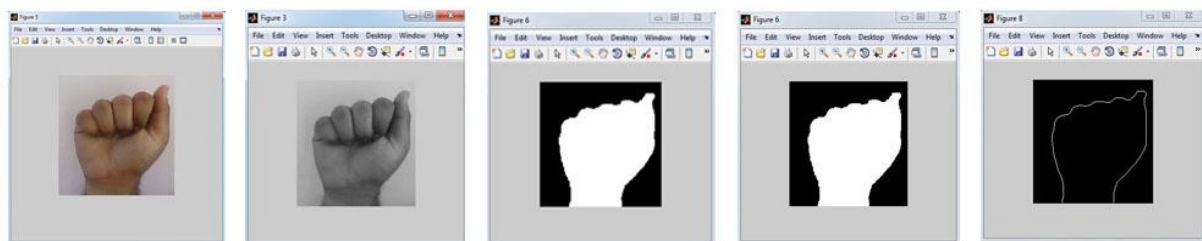
Fig.4 Outputs of pre-processing, segmentation and edge detection
