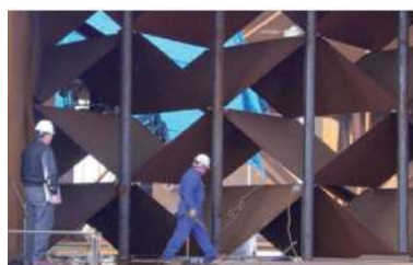
SMV mixer for optimized NO x removal (Sulzer, Inc.)
