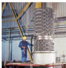
SMR-type heat exchanger for fiber cooling processes (Sulzer, Inc.)
