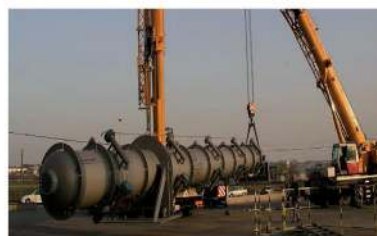
SMR reactor for polystyrene synthesis (Sulzer, Inc.)
